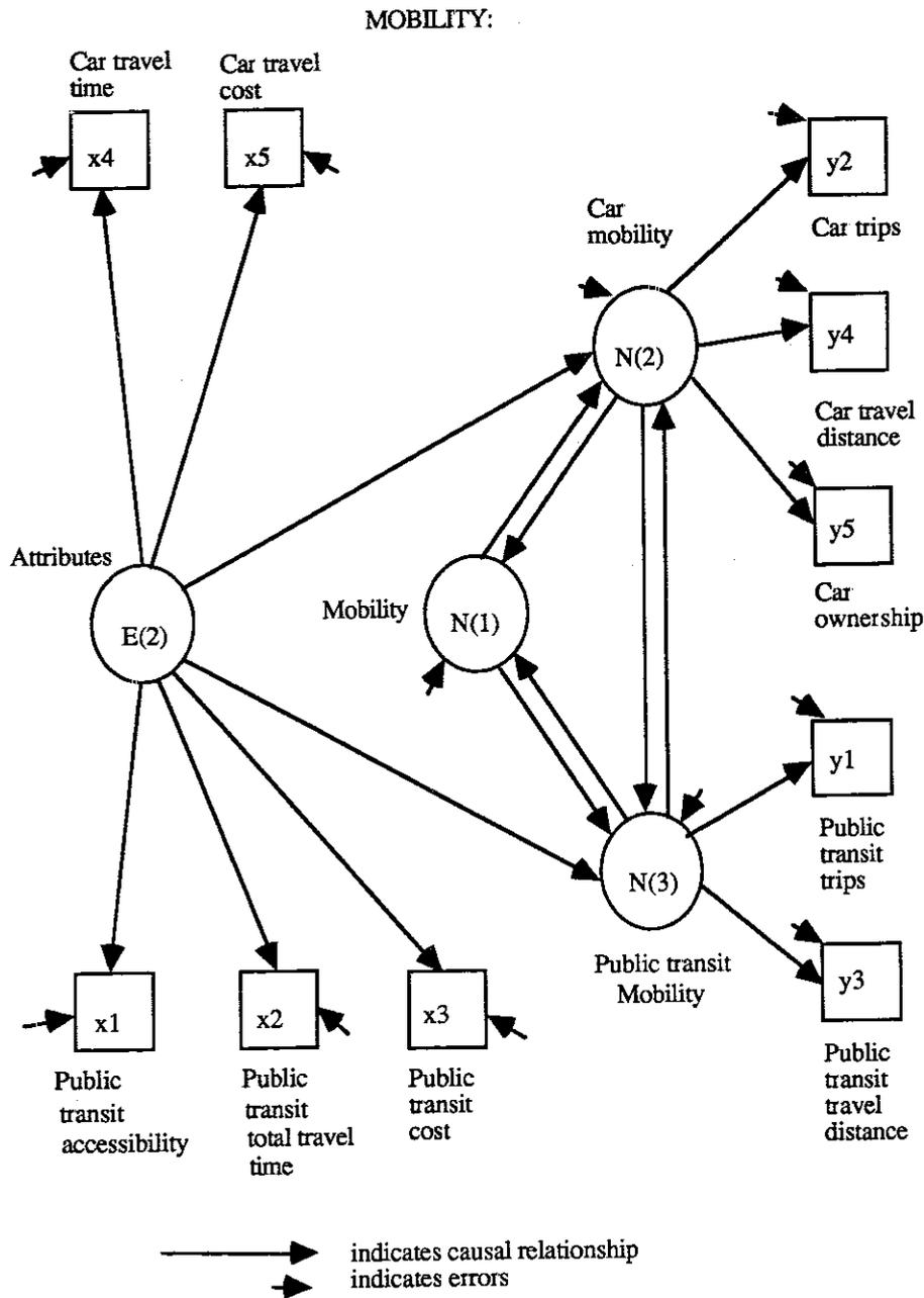
Figure 3 Components of the measurement model: mobility sub-model with assumed observed variables for each latent variable
