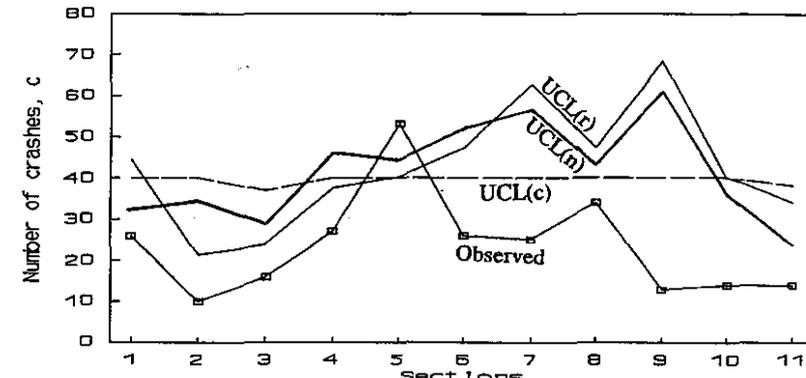
Figure 3. Crash control chart of the SQC method and of the non-distributional method, at 0.99 probability.
