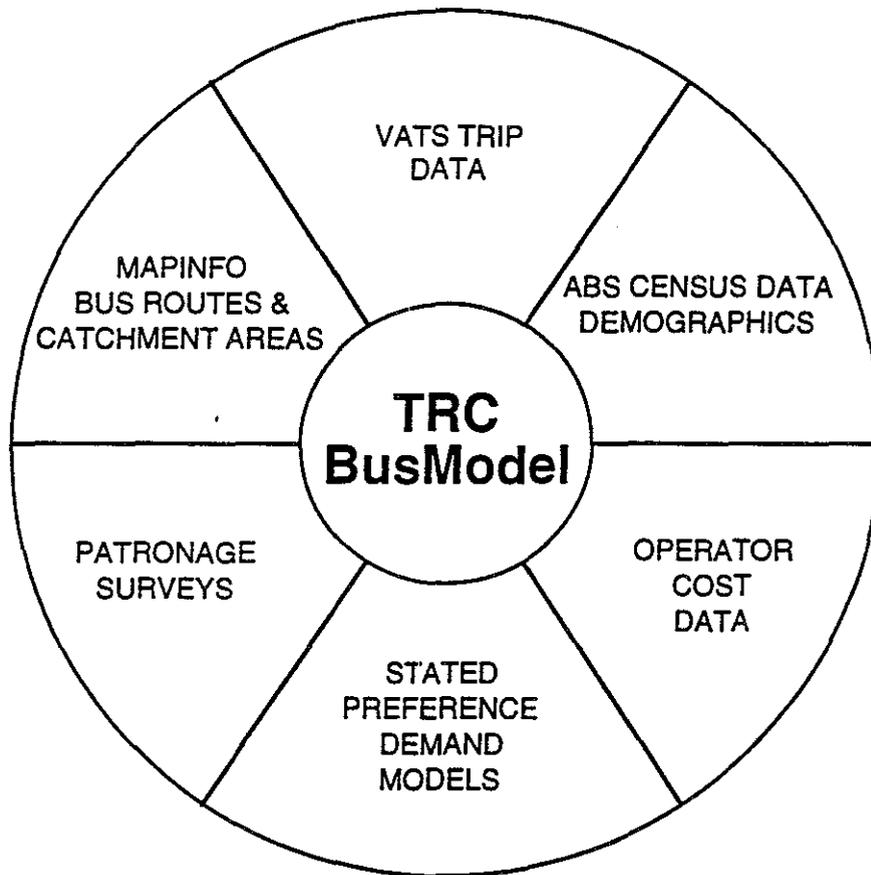
**Figure 4 Data Sources Supporting the TRC Bus Model**
