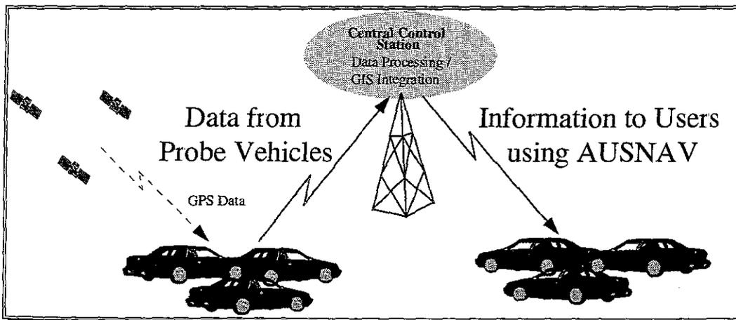
Figure 1 Schematic of Real Time Monitoring System
