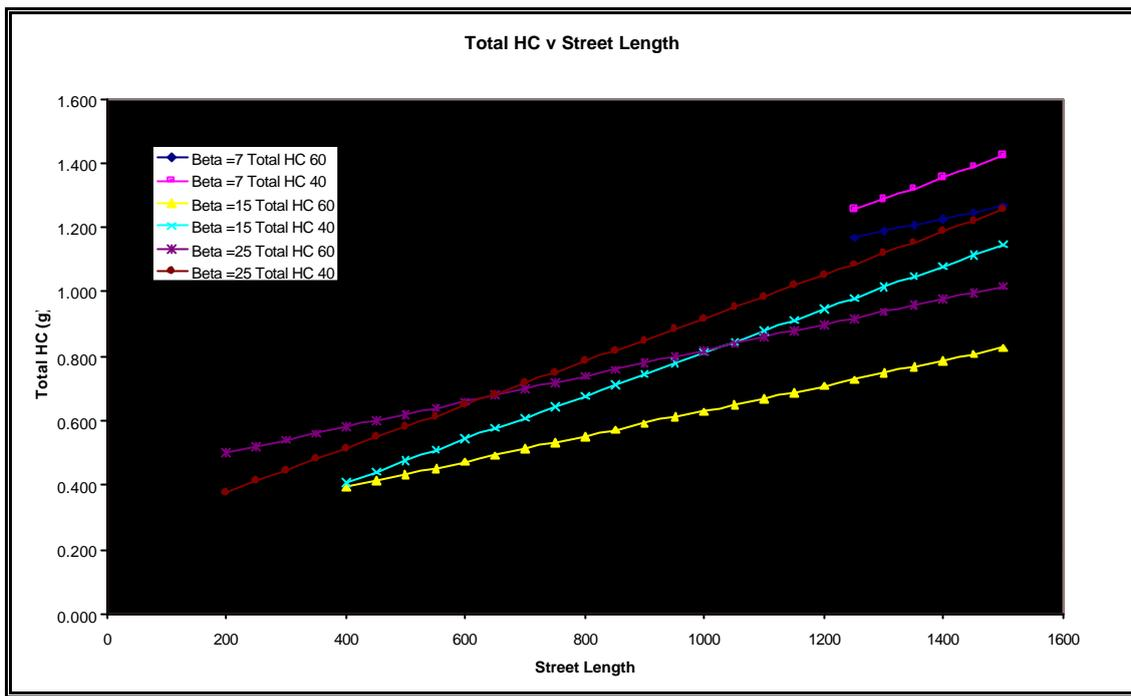
**Figure 7. Total HC emissions and street length, showing crossovers at 390 m (Scenario 2) and 620 m (Scenario 3)**
