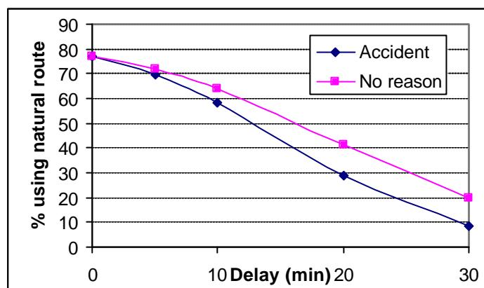
**Figure 1 The effect of delay time on proportion using the natural route**
