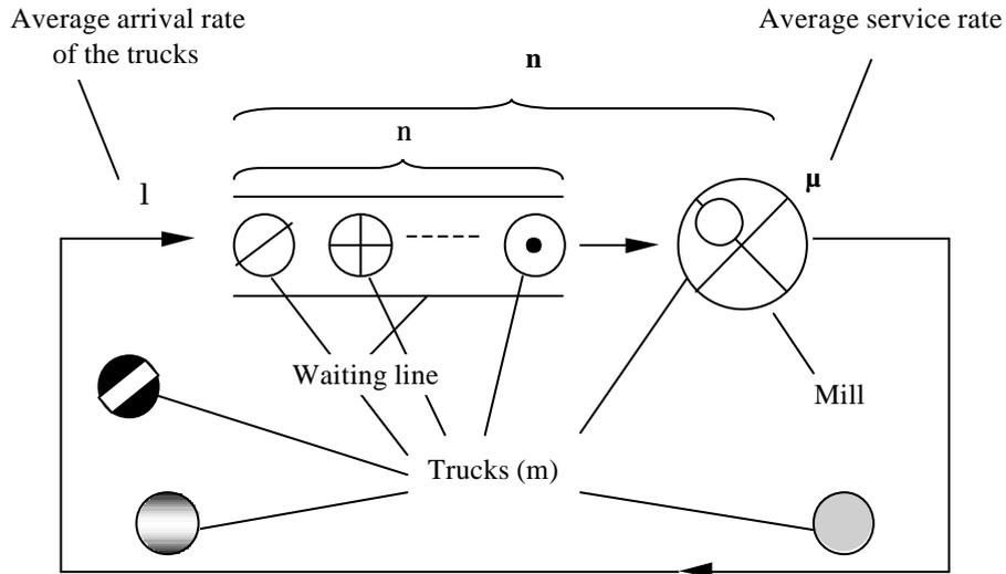
**Figure 1 - Single server, finite-population queueing system– closed circuit system**
