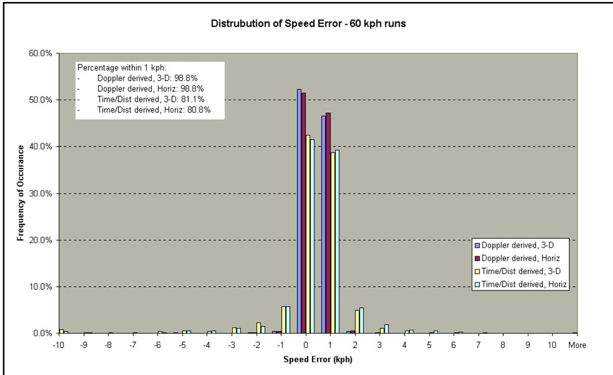
**Figure 7. Spread of error associated with GPS-derived speed**
