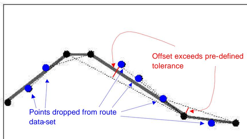
**Figure 9. Diagrammatic representation of the route-filtering algorithm**
