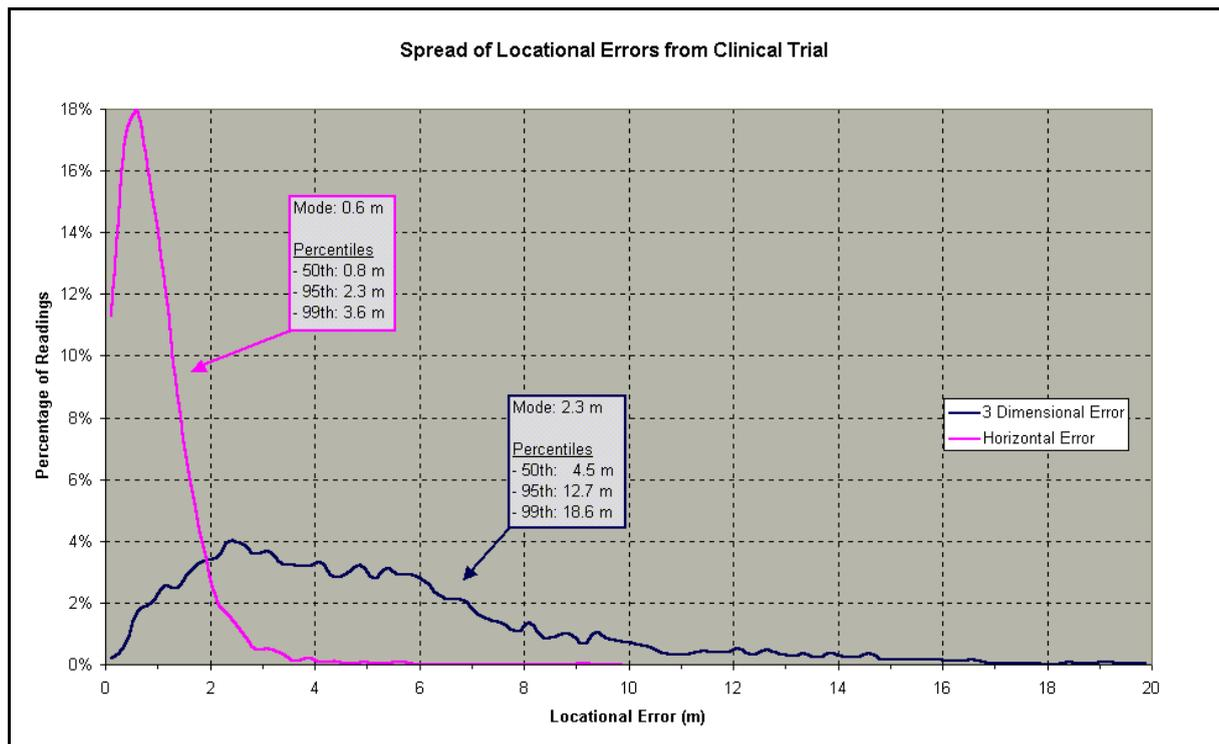
**Figure 4. Typical Locational Error from GPS without SA**
