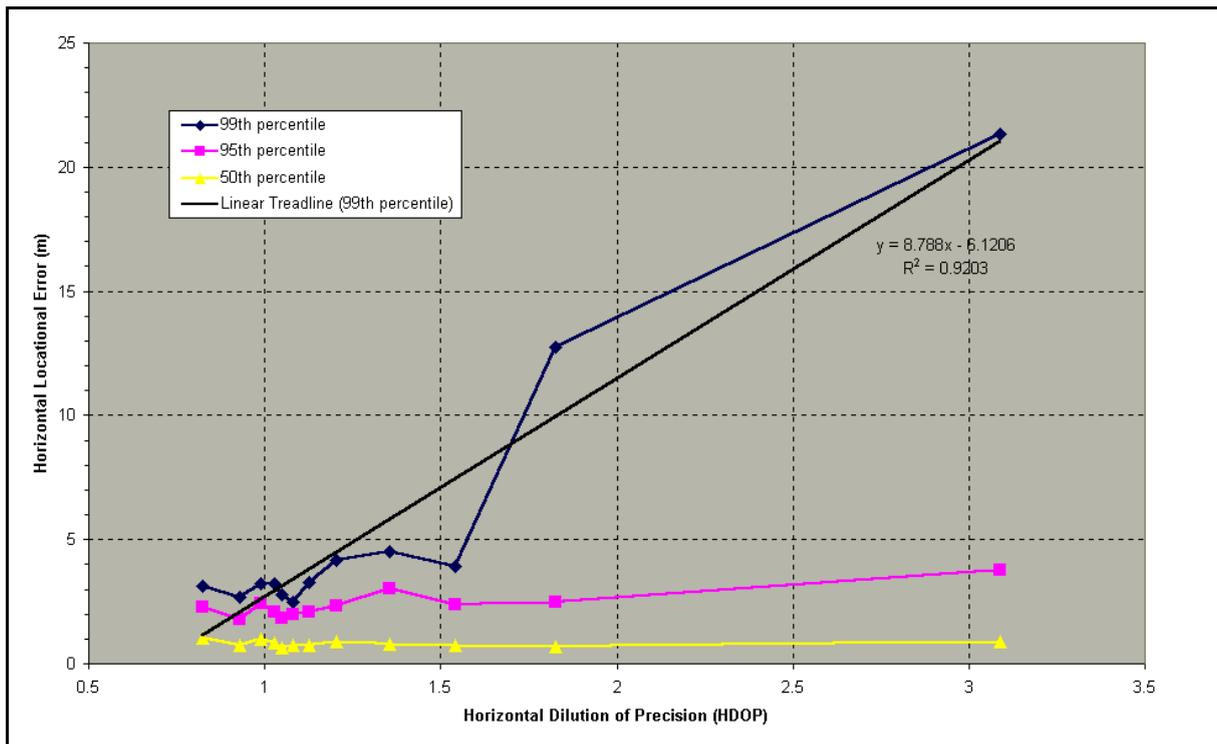
**Figure 6. Horizontal Locational Error Percentiles by HDOP**
