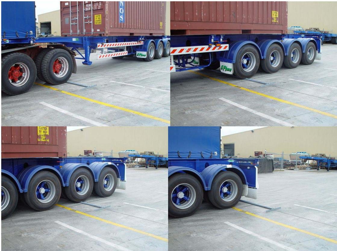
**Figure 5** Detail of progression of combination over the 50mm pipe for the bump test.
