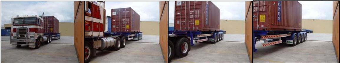
**Figure 4** Showing progression of combination over the 65mm drop between slab and apron
