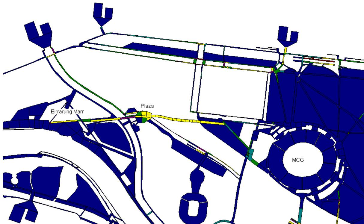
Figure 5 Level of service snapshot at 6:30pm for the Option 11b design
