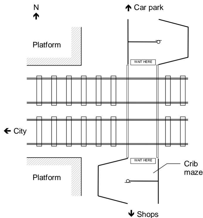
**Figure 3: Layout of the trial crossing**
