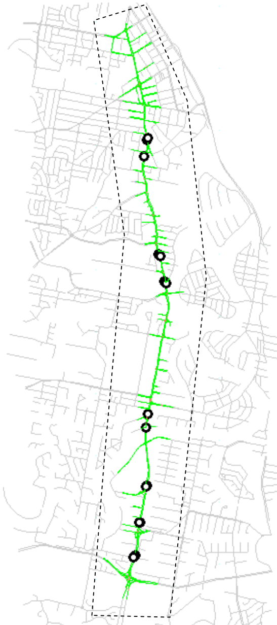
Figure 4(b): Schematic of Bundall Road AIMSUN Model
