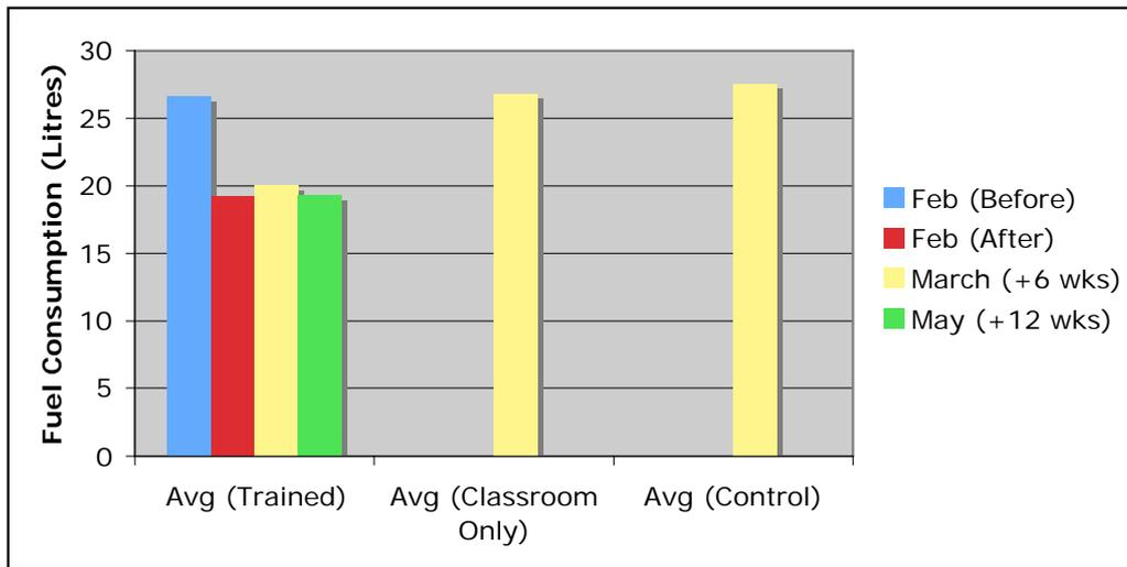
Figure 3 – Field trail results: Fuel consumption
