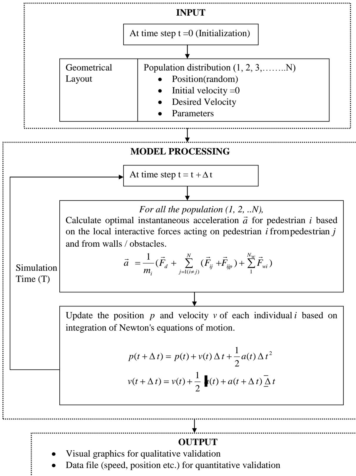
Figure 1: Flow chart of simulation program
