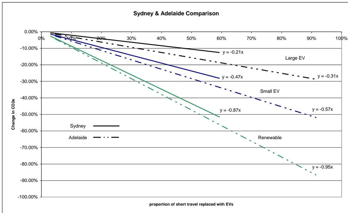
**Figure 7: Percentage change in CO<sub>2</sub> emissions for the uptake of electric vehicles in Sydney and Adelaide**
