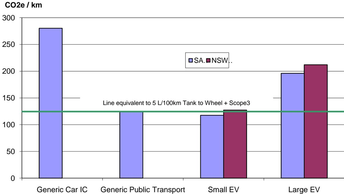
**Figure 6: Comparison of emission factors by mode, including a generic value for public transport**
