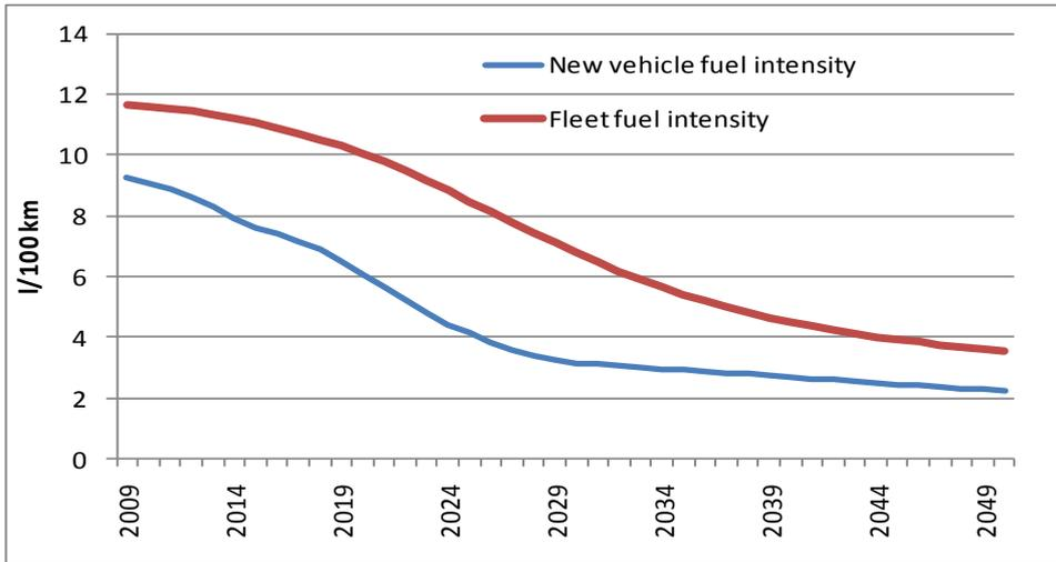
**Figure 9: Resulting light vehicle fleet aggregate fuel use**
