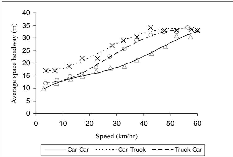
Figure 3. Speed-time headway observed in real traffic.
