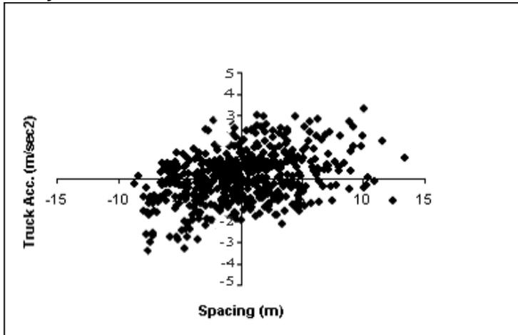
Figure 8 shows the relationship between the heavy vehicle acceleration and its spacing for freeway leader vehicles and heavy vehicles (Lead vehicle in Figure 1). The spacing (the direct distance between the front bumper of the heavy vehicle and the front bumper of the lead vehicle) measured with respect to the heavy vehicles is defined as follows:
