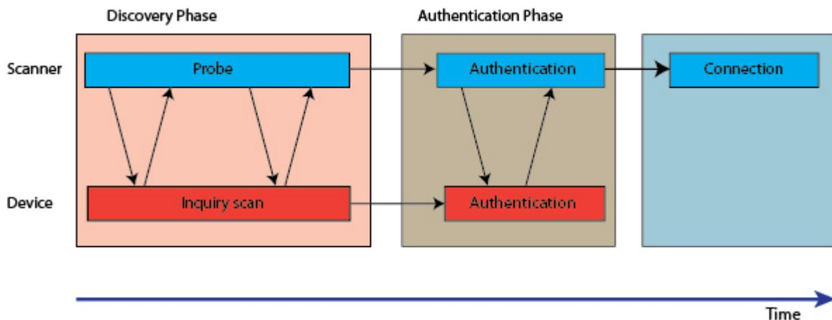
Compared to the BT device (recommended) inquiry time of 10.24 seconds, Wi-Fi has a total inquiry time of as little as 8ms. This allows detection of devices every second, allowing vehicles that travel through a zone to be detected at a much quicker rate.
