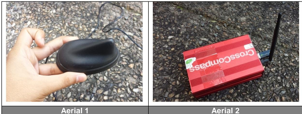
To determine the range of the aerials, the device was set up with a laptop to monitor the detected devices in real time. A controlled device, with a known MAC-ID was monitored as it moved away from the scanner. When the device was unable to be detected by the scanner, the device was deemed to be out of range. The distance between the device and the scanner was then measured using a GPS based device, determining the range of the attached aerial. This process was carried out with both aerials.
