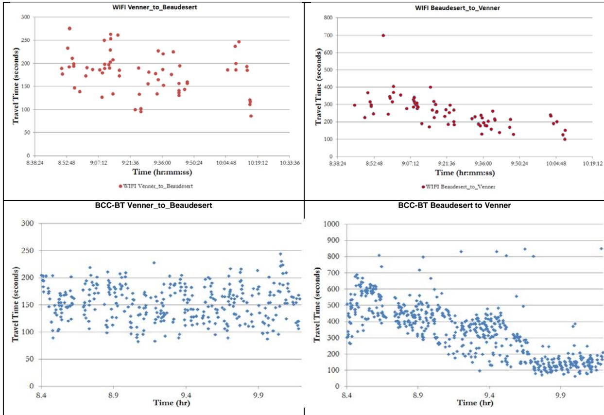
The above graphs illustrate the variation in travel times in both inbound and outbound directions. The top graphs represent the travel times determined using WMS and the bottom graphs represent the travel times determined using the BCC-BT data.
