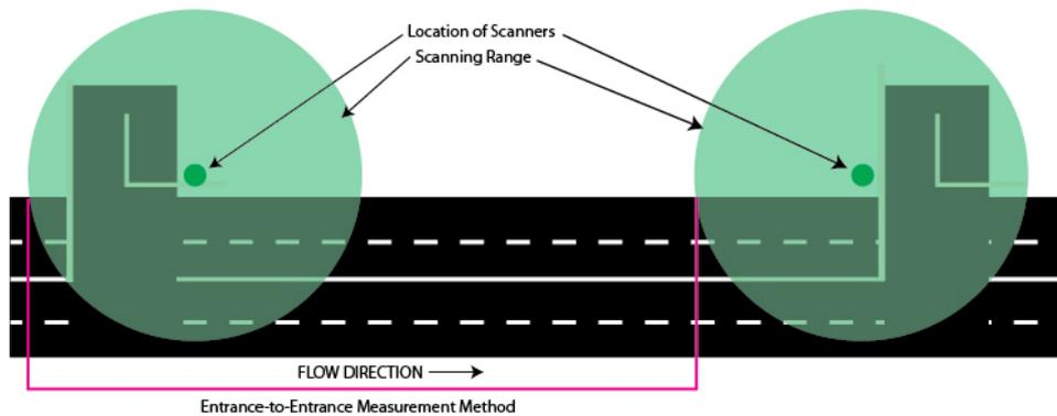
The vehicles entering the first sensor range may actually be stopped at the intersection, with dwell time for a stop signal. The amount of time that the vehicle is stationary depends on the level of congestion and the phase time of the intersection. If traffic is congested along the road after the first intersection, dwell time may increase in the range of the scanner.
