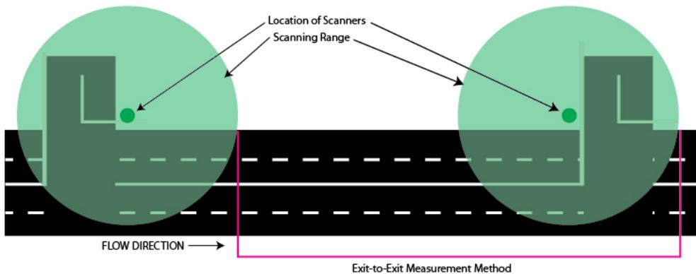
Traffic engineers use either method for traffic analysis. However for the purpose of this analysis, exit to exit method is used. In the process of filtering out multiple MAC-IDs from the original data set, only the last occurring instance of the MAC-ID was used in the analysis.
