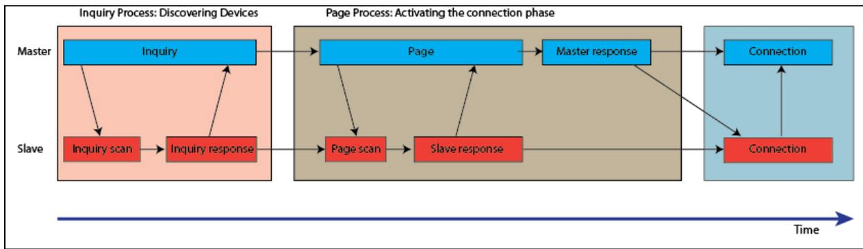
The inquiry phase of connecting BT devices may take 10.24 seconds, as the scanner has to scan 79 frequencies that are available to BT, between 2.402GHz and 2.48GHz. The frequencies of BT are separated into 32 channels, made of two 16-channel subsets called trains. Scanning of each of the trains takes 0.1 seconds and each train is scanned 256 times to provide adequate collection time from other BT devices (Vo, 2011).
