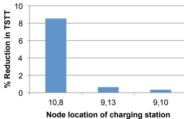
Two examples where multiple charging stations have little system impact, (9,13) and (9,10) are represented in Figure 5. Additionally, installing charging stations at nodes 10 and 8 reduced TSTT less than installing a single charging station at node 6 or 7. This further supports the need for assignment models which account for user behaviour when comparing charging infrastructure design alternatives.
