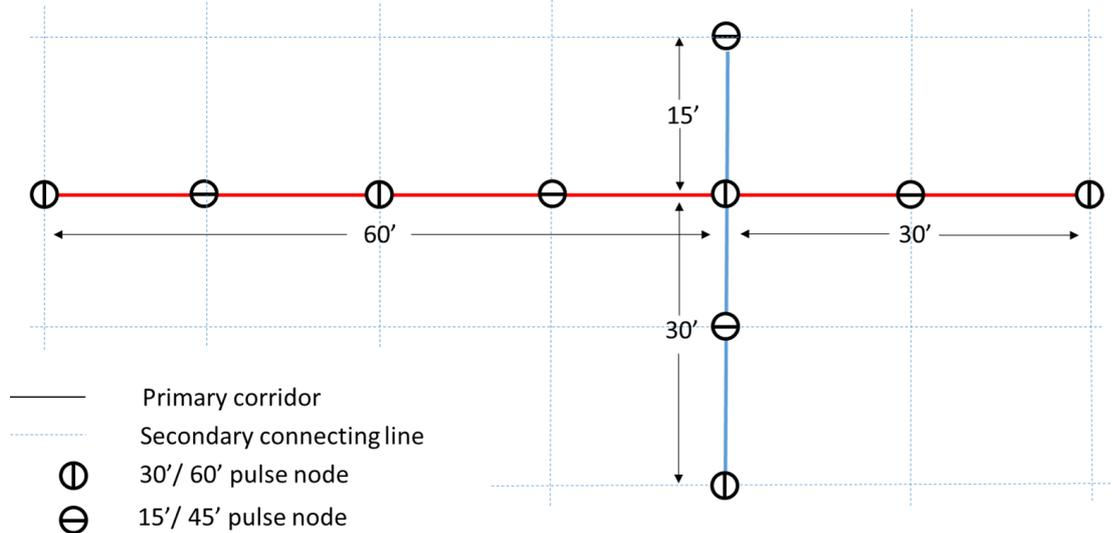
The simplified example in Figure 1 demonstrates what such a network might look like. It is a 30' interval network with two primary lines intersecting at a hub. The round trips are 3 hours for the red line and 1.5 hours for the blue line. Inbound and outbound vehicles cross at intermediate nodes, creating opportunities for convenient connections with secondary lines.
