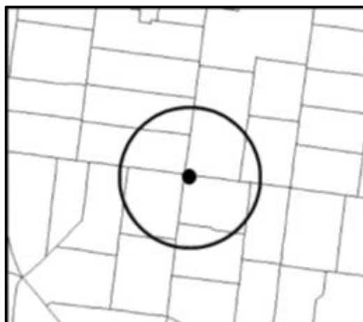
Figure 1 - Example of catchment with transit station at centre overlying SA1 shape file in MapInfo
