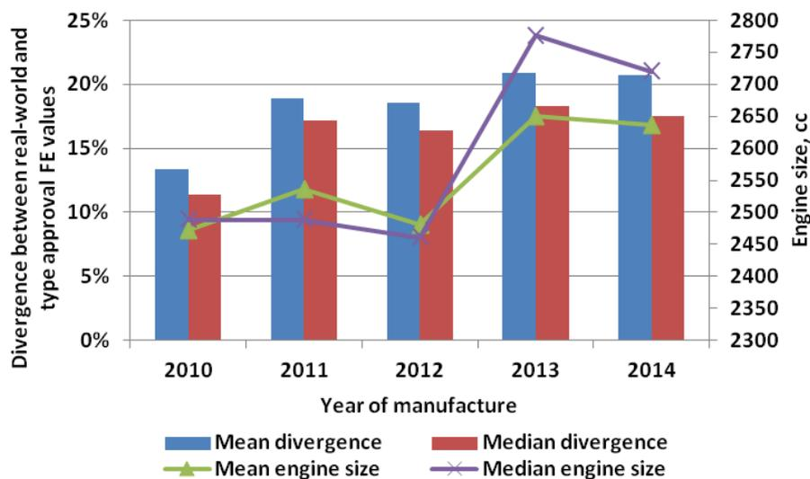
As noted above, those light diesel vehicles made in 2013 and 2014 have a larger engine size on average than those made in earlier years. Our research (Section 3.2) shows that the divergence between real-world and type-approval FE values is smaller for vehicles with larger engines. Therefore, the apparent increasing divergence trend with the YOM for diesel vehicles is less pronounced than that for petrol vehicles, where mean engine size is similar for different years of manufacture.
