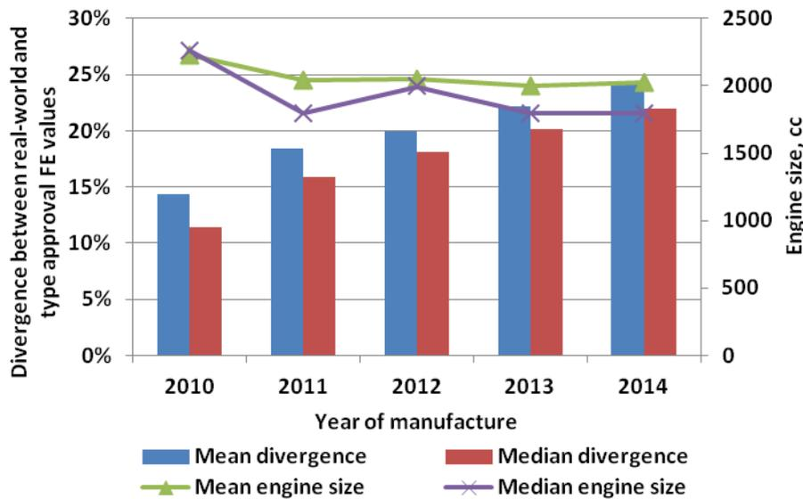
**Figure 10: The divergence between real-world and type-approval (NEDC) FE values vs. the year of manufacture for light diesel vehicles**
