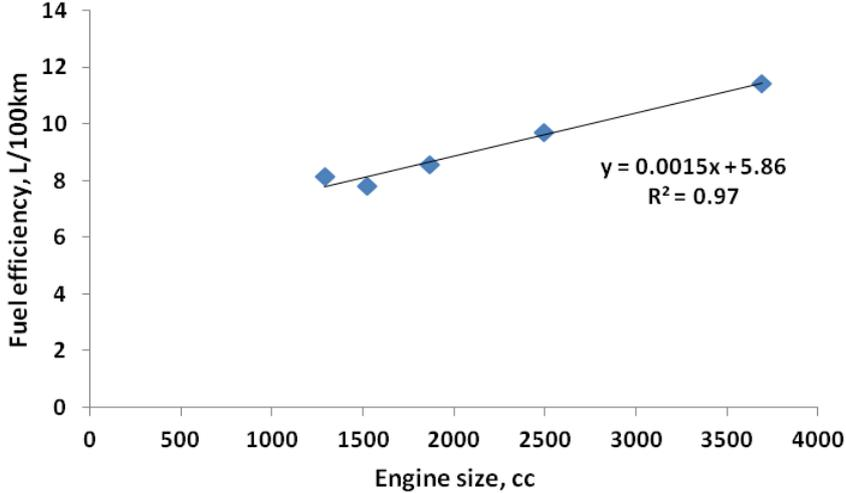
As seen in the box plots in Figure 2, FE values of individual light petrol vehicles are widely distributed. This is normal, as the FE of a vehicle is affected by many factors, such as vehicle technology, driving style (frequency of acceleration and deceleration, and speed), road conditions, geography, weather conditions, and the use of air conditioning. On the other hand, the trend for increasing fuel use with increasing engine size can be still seen clearly in Figure 2.
