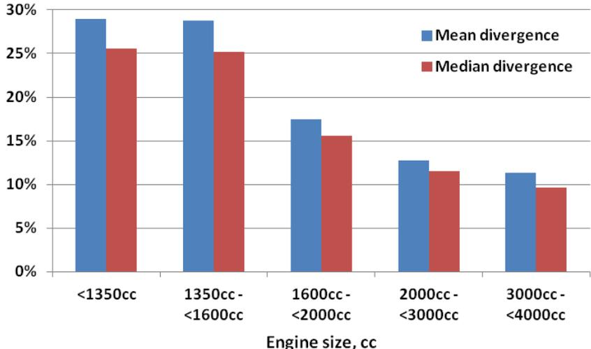
**Figure 5: The divergence (vertical axis) between real-world and type-approval (NEDC) FE values of the light diesel vehicles (all analysed vehicles included)**
