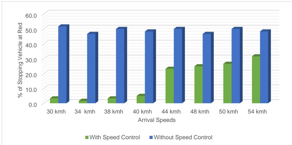
Figure 5: Relationship between vehicle arrival speeds and stopping at red
