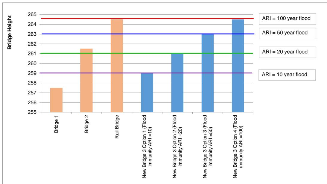
The proposed Bridge 3 can be raised to a height that would stand for either 1 in 10, 20, 50 or 100 year flood. Typically a higher design standard would mean a higher capital cost.
