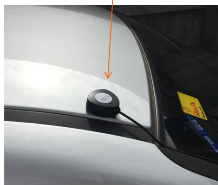
Figure 3: Mounting of Racelogic VBOX Sport (left) and its external antenna (right) Suction cup mounting on the windscreen Magnetic mounting of the external antenna
