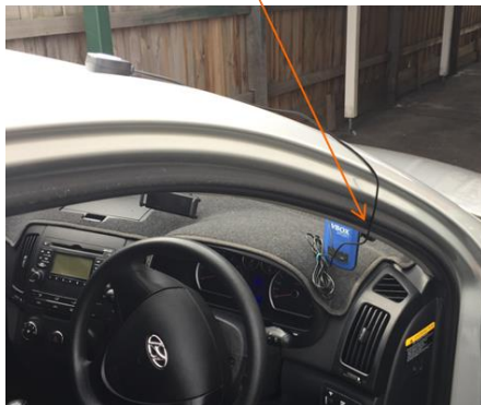
Figure 3: Mounting of Racelogic VBOX Sport (left) and its external antenna (right) Suction cup mounting on the windscreen Magnetic mounting of the external antenna
